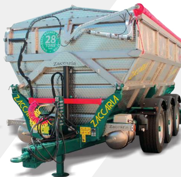
Pneumatic PVC side covering. Right side. Activation by remote control.
