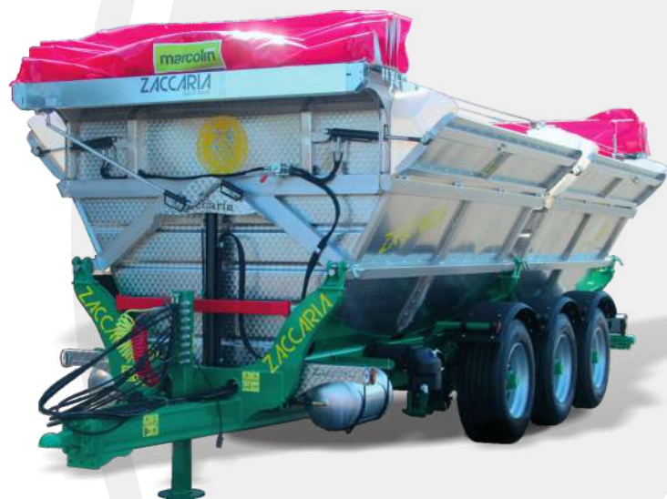
Front sliding PVC manual covering with crank
